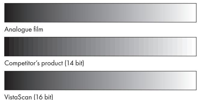
The greyscale gradation of the VistaScan image plate enables depiction on a par with that of film
