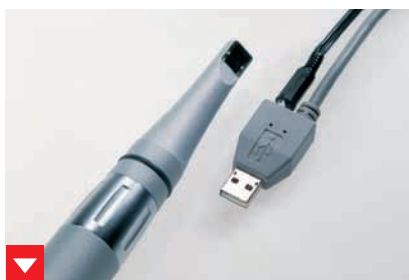
The power supply of the VistaCam Digital is ensured with a separate and direct power supply at the USB plug in accordance with MPG.
